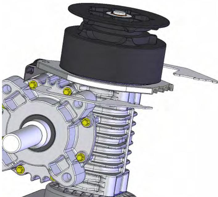
Take the pair of dovetail body brackets (see picture to the left) and move together, placing them around the body of the gearbox.
