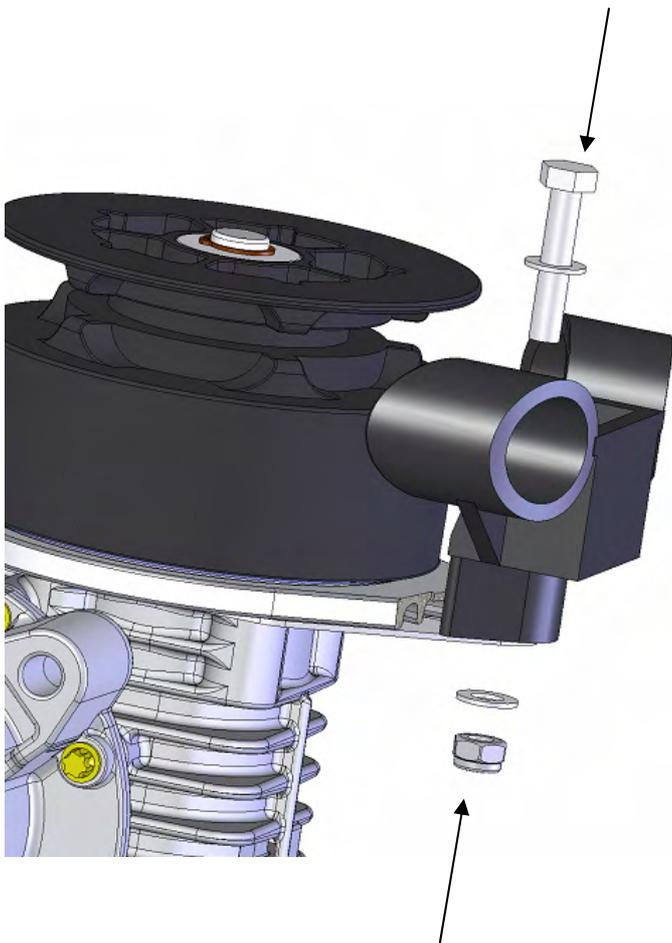
Place the packer and the chain guide over the exposed hole in the dovetail brackets. Insert the Hex head bolt, through a washer, then into the assembly. Fasten underneath with a washer and nylon lock nut.
