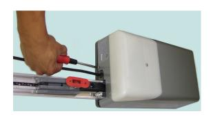
2. Remove the GTS cover by pulling in the directions of arrows as shown in the figure
