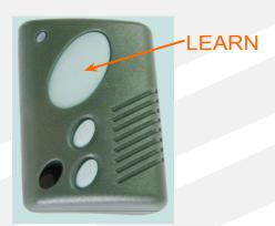
Note: To reset the receiver press and hold the learn button (2.) for 12 seconds. This will erase all handsets from the memory. This is recommended if a remote has been lost or stolen. Any other handsets previously used will need to be reprogrammed by following steps 1, 2 and 3 above.
