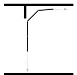
Sectional doors – comprise of a number of rigid sections that are hinged together and move vertically in the opening, then horizontally along the ceiling, guided by tracks and counter-balanced with springs. Commonly used on new houses where a pattern or style is required to match the style of the house. These doors can be made of steel, wood and other materials. The B&D Panelift® range offers a broad selection of styles and colours.
