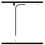
Flex-A-Door® doors – comprise of a durable Roll-A-Door® curtain, fitted on a curving track, which slides from a vertical position up into a horizontal position, close to the ceiling. Especially suited to applications where there is not the headroom for a roller door or, where a smoother, easier to use solution is required to replace an existing tilt door.
