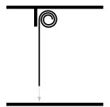
Roller doors – comprise of a ribbed steel curtain that moves vertically in the opening, and rolls up around a drum, guided by tracks and counterbalanced with springs. They are particularly suitable for garages and sheds where there is plenty of headroom above the opening and where a traditional look is required. The B&D Roll-A-Door® is the original roller door, with 50 years of added innovation and improvement.
