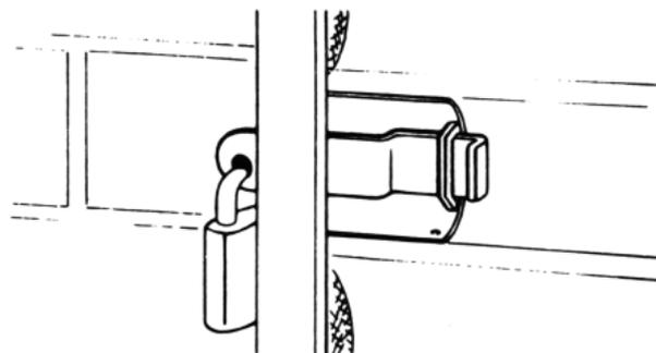
With door fully closed check that bolt slides through guide. Adjust hole if necessary.
