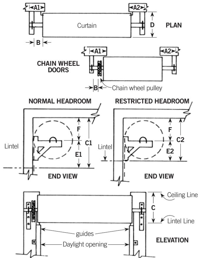
**NOTE:** Hand operated doors up to 2400mm high, the bottom rail will hang 65mm below lintel. For doors over 2400mm high bottom rail will be level with lintel.
