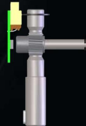
At the end of the **timing shaft** is a small magnet positioned a few millimetres over a **sensor**.
