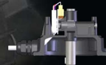
Inside the sealed orange cover, the **M-ALPS' worm drive shaft** then rotates a **helical geared timing shaft**.
