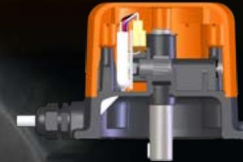
The opener's output drive shaft has a key way into which the **M-ALPS' worm drive shaft** is slotted. When the opener is driving, the limit assembly is turning.
