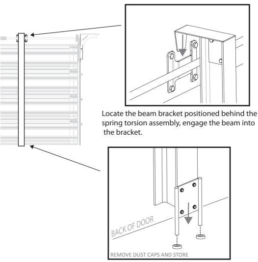
Locate the base pins into the plastic sleeves at the base of door.
