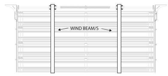
Depending on the width of your Centurion C2 Safe door, you will have one, two or three wind beams installed alongside your garage door.
