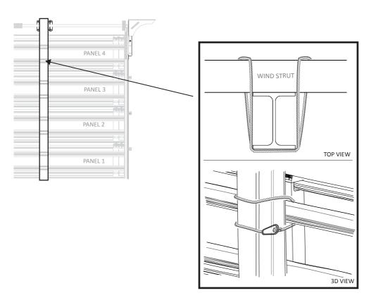
Ensure all wire cables are fitted and attached at each beam and garage door connection point. (Two cables per door panel for each beam)
