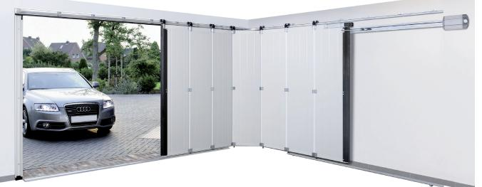
The side sliding sectional door has been developed for use in applications which have limited head room. This innovative solution consists of 42mm insulated panels and operates with a trip free threshold. Available in Micrograin, Duragrain and the Silkgrain finishes, this door can be automated and has the convenience of a custom handle for easy pedestrian access.
