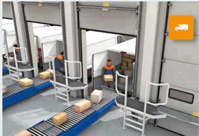
Vans are loaded at floor level. For this purpose, the door is opened completely including the bottom section
