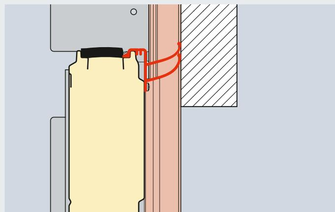
Lintel fitting with ThermoFrame
