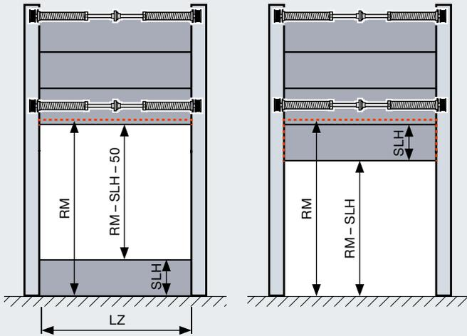
When the coupled door is opened (right figure), the bottom section with the catwalk remains in the top part of the door opening.
