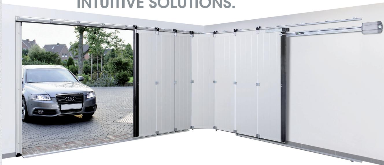
The side sliding sectional door has been developed for use in applications which have limited head room. This innovative solution consists of 42mm insulated panels and operates with a trip free threshold. Available in Micrograin, Duragrain and the Silkgrain finishes, this door can be automated and has the convenience of a custom handle for easy pedestrian access.
